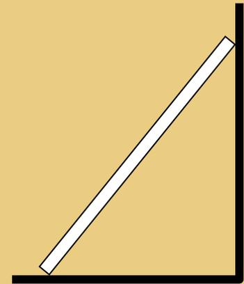
Is it possible for the ladder to be in equilibrium if the floor is frictionless? In other words, as long as the friction between the wall and the ladder is great enough, will the ladder stay in place?
