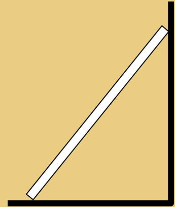
Is it possible for the ladder to be in equilibrium if the wall is frictionless? In other words, as long as the friction between the floor and the ladder is great enough, will the ladder stay in place?
