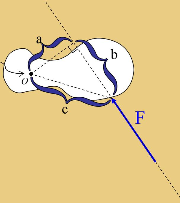
Which distance in the diagram above is the moment arm of the force with respect to rotation about  $O$ ?
