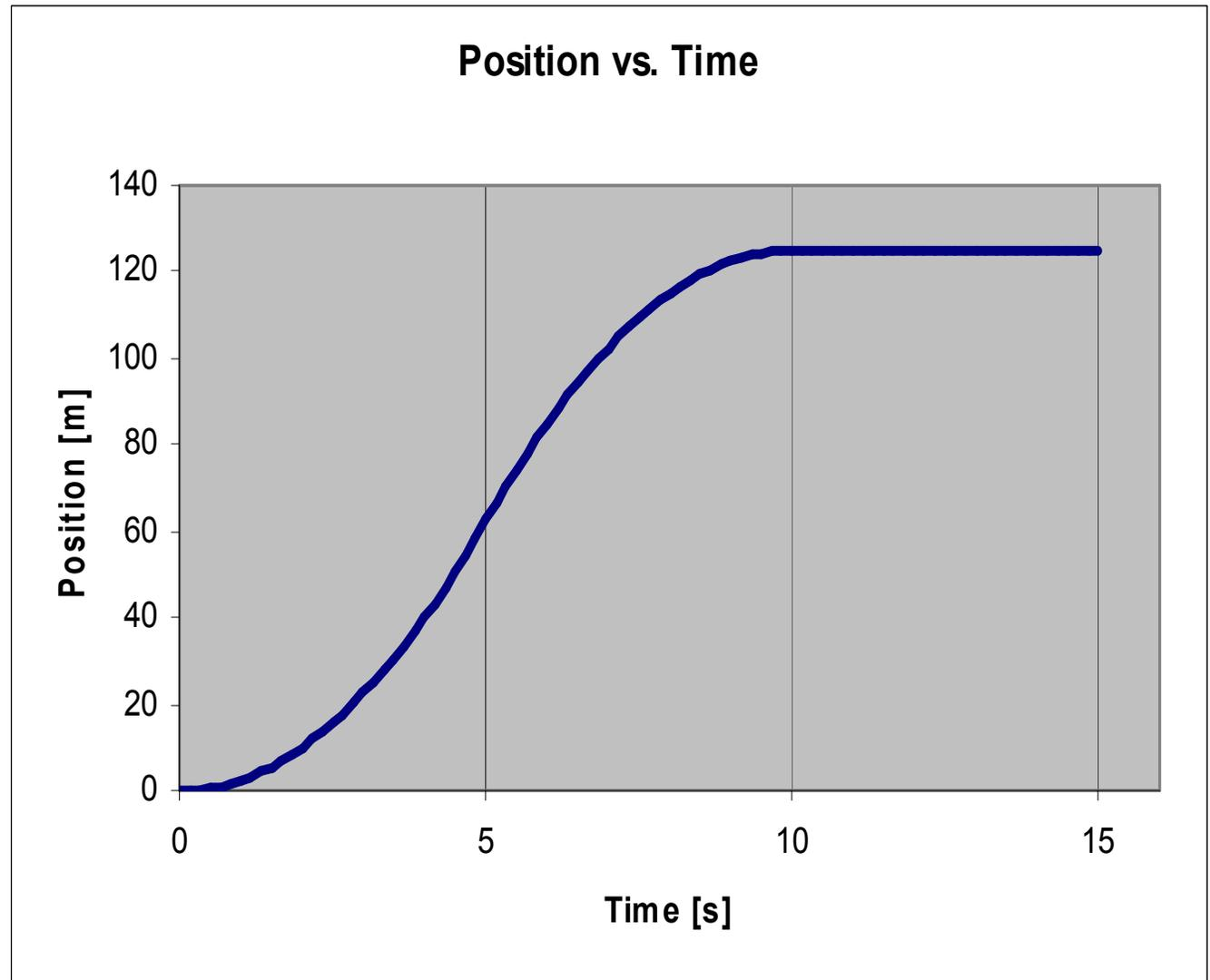
During which time interval is the car always at rest?
